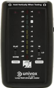
Univox FSM Basic or equivalent field strength meter
