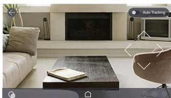
1. Touch the screen, and the Pan/Tilt Control button is displayed on the screen.
